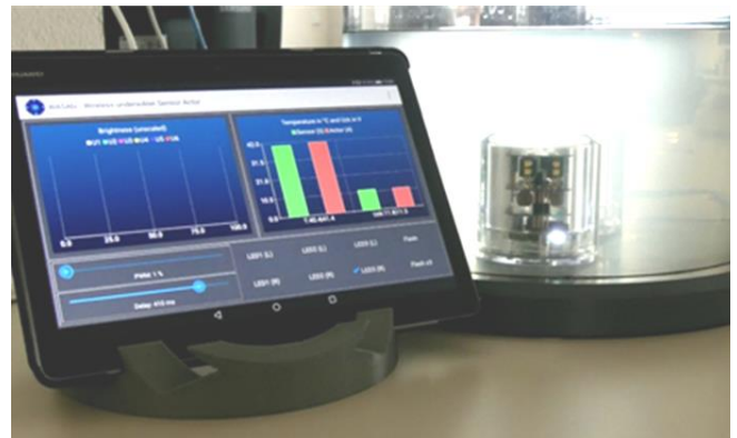
Fig. 2. WASABI - Wireless underwATER Sensor Actor with Bidirectional data transfer and “plug-free” power transmission consisting of: water tank, two sensor-actor modules (switchable), inductive power supply and processing unit (tablet)
