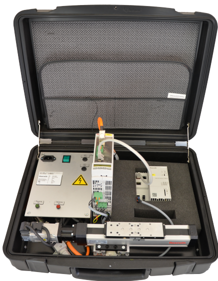
Fig. 2. Ball screw drive with Rexroth control as machine component
