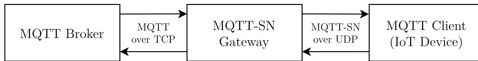
Figure 2.4: Architecture components used by MQTT-SN: In addition to an MQTT broker, MQTT-SN requires a gateway that translates between its clients, which speak MQTT-SN over UDP, and the broker, which speaks MQTT over TCP. The gateway may be integrated with the broker or it may be a standalone component, as shown here.
